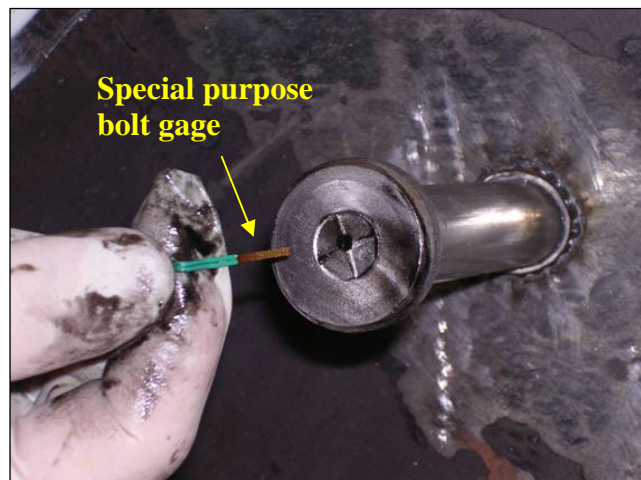
Figure 3.8: (a) Stud gage installation
