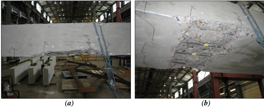
Figure 5.7: Complete haunch separation as seen from (a) the side view and (b) underneath the specimen
